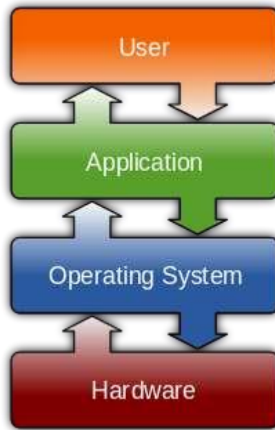
Fig show: A layer structure showing where the operating system software and application software are situated while running on a typical desktop computer.
